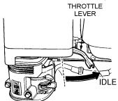
Figure 14. Throttle Lever (Idle)
